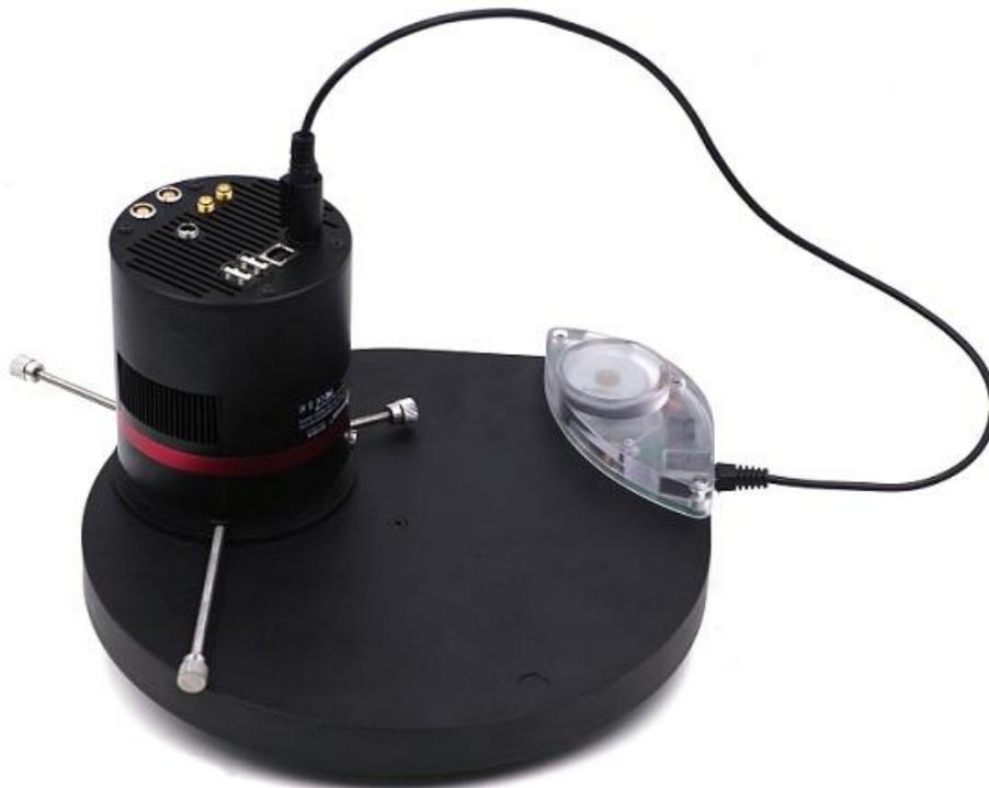
First, you need to stick QHY29M into QHYCFW2-L as shown in the picture above. Then you should screw those three bolts in. At the first time you screw bolts, you may find it a little bit difficult to screw in, in this case, please make sure that the bolts are pointing towards the center and apply a little bit more of force. Finally, you should connect your QHY29M with QHYCFW2-L by using DIN4/RJ11 cable, which is included in the box.
